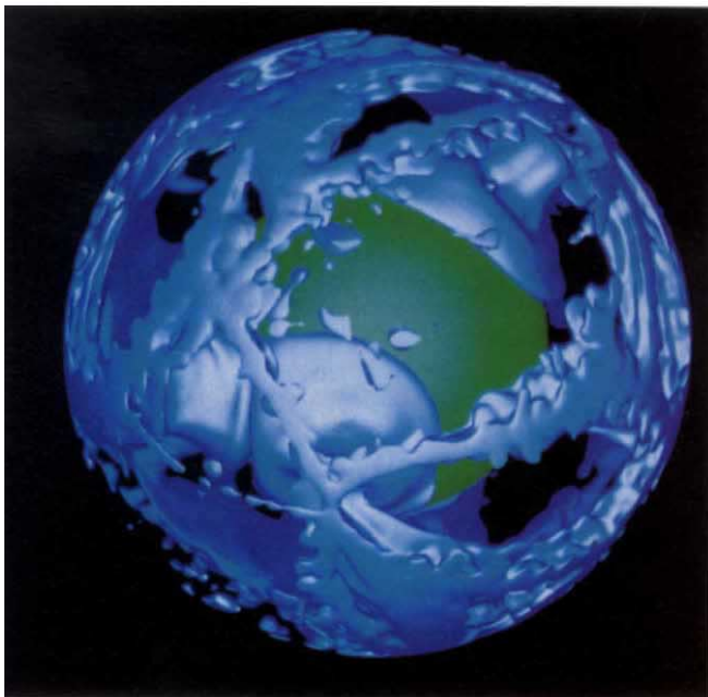
FIG. 1 Cold downwellings for final frame of simulation. Blue surface is an isocontour showing where the temperature is 110 K lower than the horizontally averaged value. Green surface is the core. A network of interconnected linear downwellings is visible in the upper mantle, with three huge cylindrical downwellings in the lower mantle, spreading out into pools of cold material above the core-mantle boundary.
