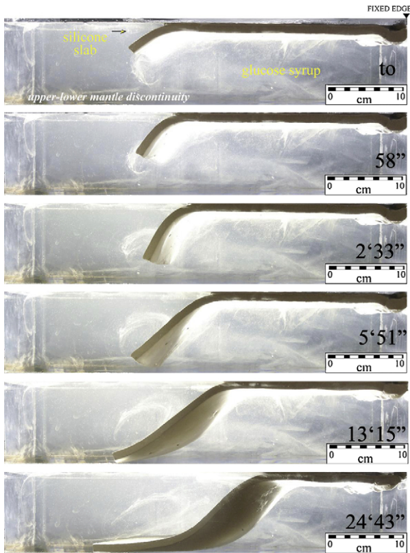
Fig. 14. Result of the laboratory experiment at 6 different times. Note that the dark visible regions represent the side view of the slab while slightly lighter parts show the central part of the slab deeper within the tank.
