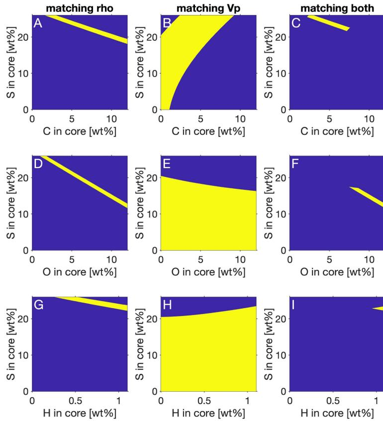
**Extended Data Fig. 3 | Matching core seismic properties in the quaternary system inside the core.** Range of core compositions in the liquid Fe-Ni-S-X (X = C, O, H) quaternary system (blue regions) that match InSight observations (yellow regions) of core density (left column, panels a, d, g), core P-wave velocity (middle column, panels b, e, h), and both properties simultaneously
