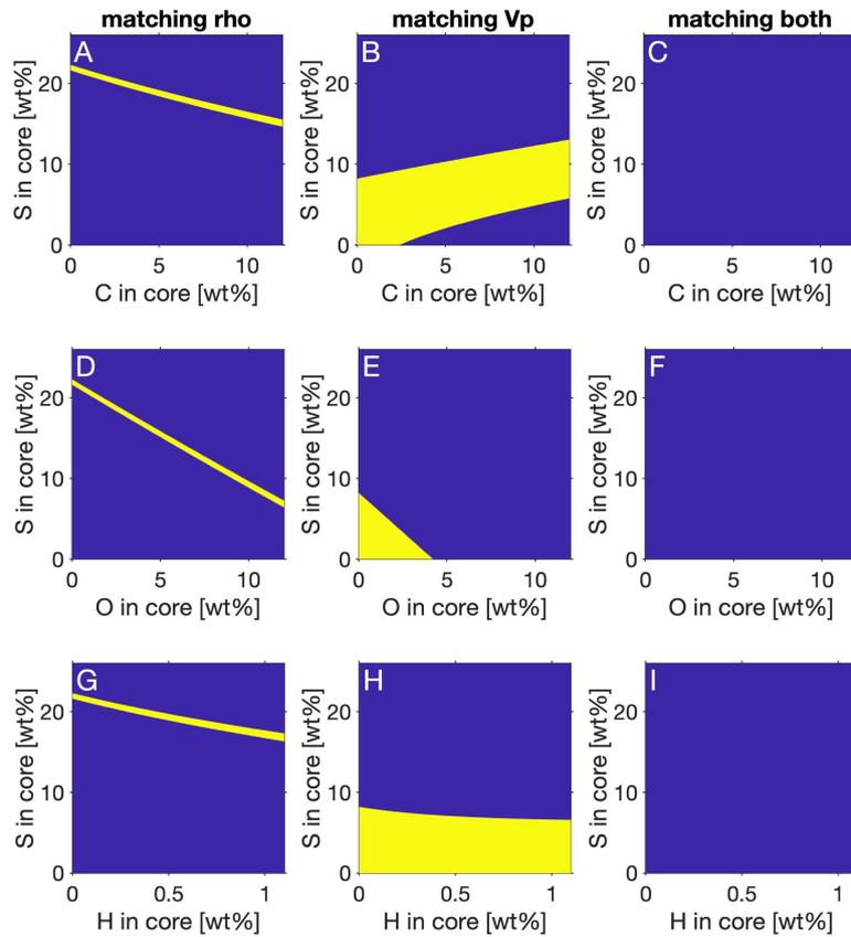
**Extended Data Fig. 2 | Matching core seismic properties in the quaternary system at the core-mantle-boundary.** Range of core compositions in the liquid Fe-Ni-S-X (X = C, O, H) quaternary system (blue regions) that match InSight observations (yellow regions) of core density (left column, panels a, d, g), core P-wave velocity (middle column, panels b, e, h), and both properties
