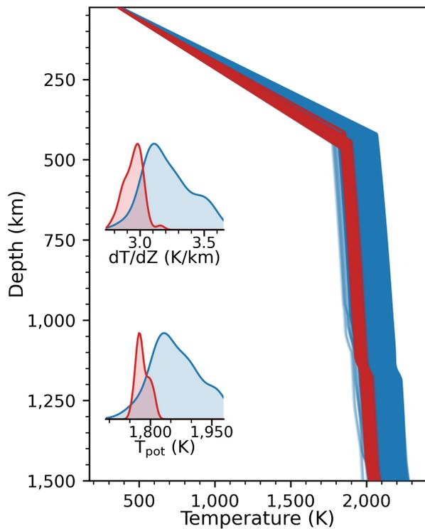
**Extended Data Fig. 5 | Martian mantle geotherms.** Inverted lithospheric and mantle geothermal profiles for high<sup>55-58</sup> (blue), and low<sup>4</sup> (red) FeO mantle compositions. The insets show the distributions of sampled potential temperature ( $T_{\text{pot}}$ ) and lithospheric geothermal gradient ( $dT/dz$ ) for high (light blue) and low (light red) FeO compositions.
