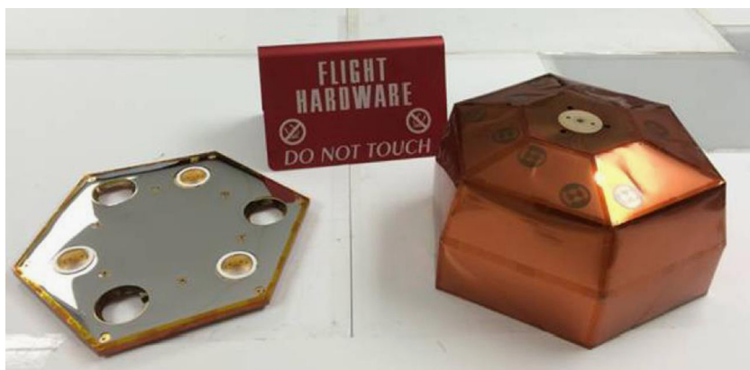
Fig. 69 SEIS RWEB (Remote Warm Enclosure Box). The width of the RWEB is \sim 355 mm and its height is 212.5 mm
