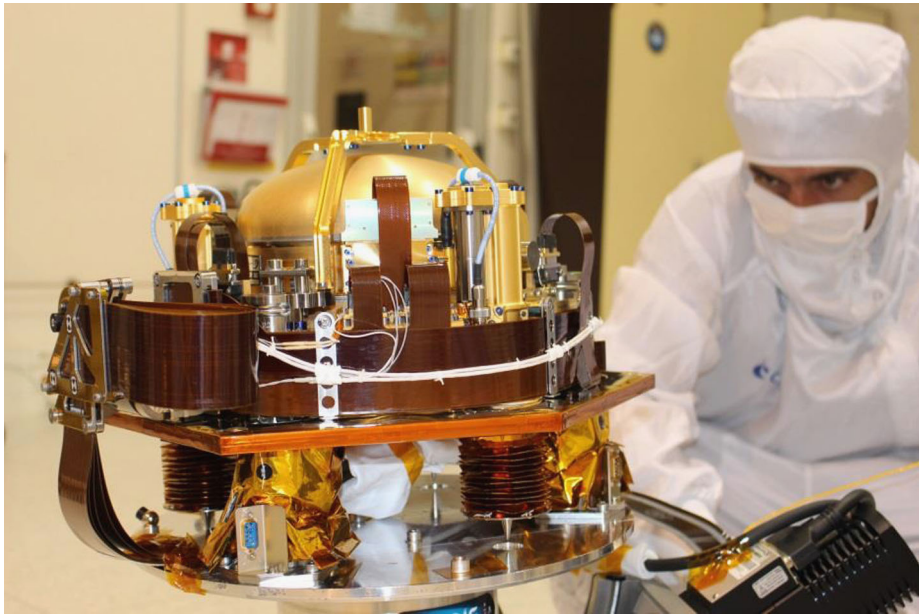
Fig. 11 SEIS Sensor Assembly (SA) without the RWB
