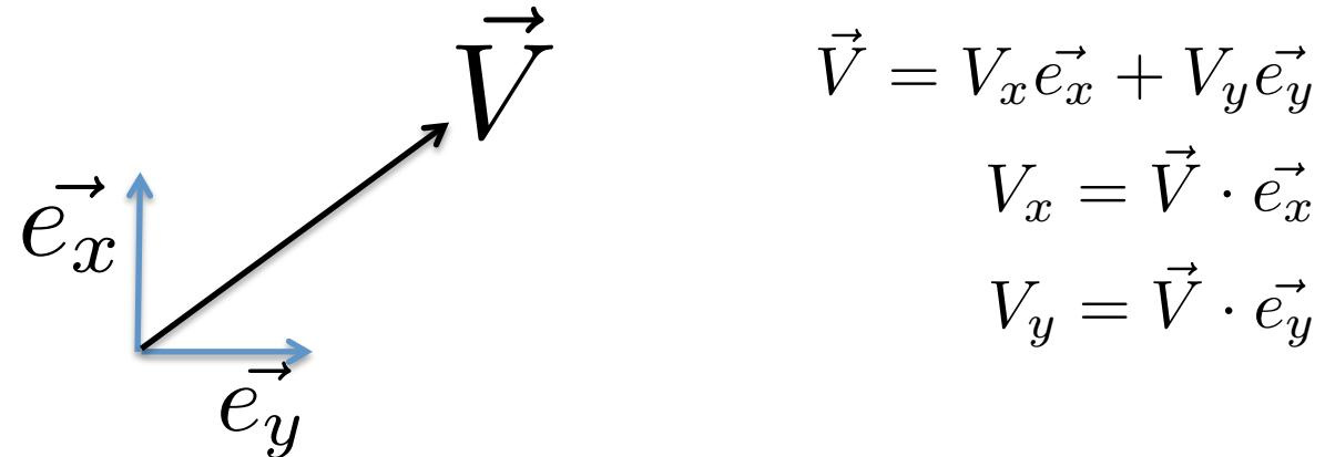
$$\begin{aligned}\vec{V} &= V_x \vec{e}_x + V_y \vec{e}_y \\ V_x &= \vec{V} \cdot \vec{e}_x \\ V_y &= \vec{V} \cdot \vec{e}_y\end{aligned}$$
